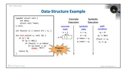
And, finally, the program's error is triggered, so DSE has identified a particular concrete input that triggers the error.
