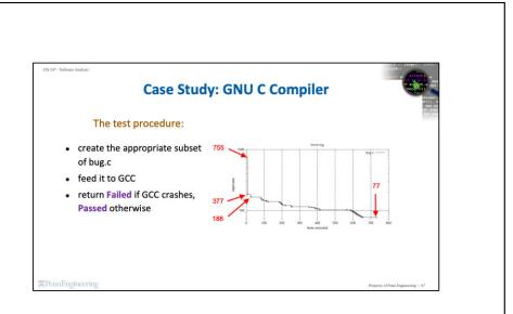
We next write the test procedure to be provided to the delta debugging algorithm. This procedure consists of three steps. First, it creates the appropriate subset of bug.c. Next, it feeds this subset to GCC. Finally, it returns Failed if GCC crashes, and Passed otherwise.
