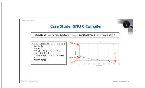
The test case now only contains the mult function: the copy and main functions have been eliminated. Reducing mult, however, takes time. Only after 731 more tests do we get a test case that cannot be minimized further. This test case only contains 77 characters.
