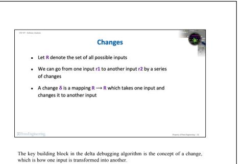
Formally, a change is a mapping from the set of all test inputs to itself. In other words, it's a function that takes a test input  $r_1$  and returns another test input  $r_2$ .
